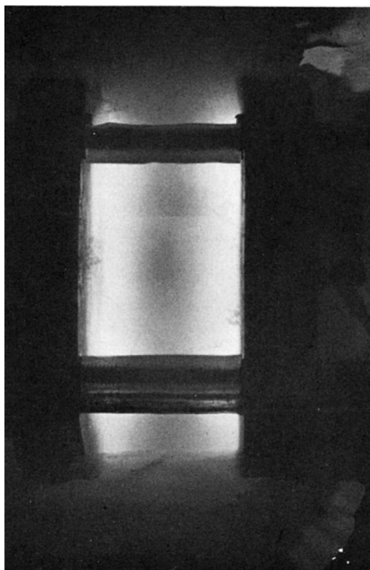
Fig. 7. Glow discharge obtained using a flow rate of 2 \text{ cm}^3 (S.T.P.)/min, p_M = 40 \text{ mTorr} , 100-W power, and magnetic enhancement.
